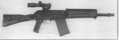
The Saiga-12C shotgun with a 580mm choked barrel, folding buttstock extended, and experimental 10-round magazine; (inset) detachable pistol grip is available option. (left) Saiga-12K shotgun, with buttstock extended, cylinder-bore 430mm barrel and a choke muzzle attachment, equipped with PO 3.5X optical sight.
